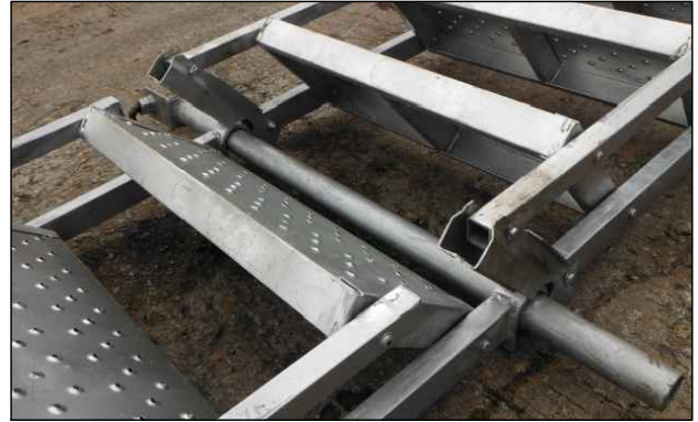
Bar-ring mechanism for installation of continuous staircases.
